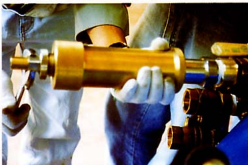
Inserting Transducers
